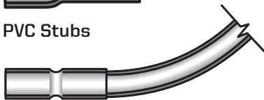
Deep Socket PVC Coupling bonded onto fiberglass elbow
