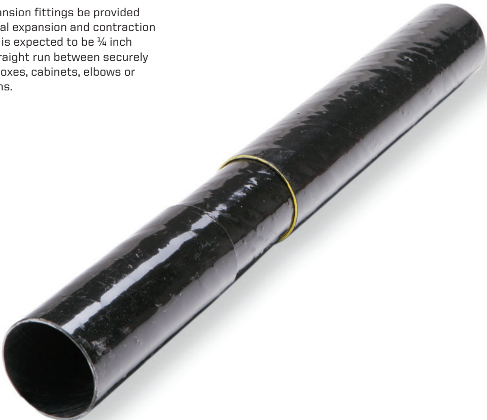
Expansion Characteristics of Champion Fiberglass Reinforced Thermosetting Resin Conduit (RTRC) Coefficient of Thermal Expansion = 5.1 \times 10^{-6} in/in/°F ( 9.27 \times 10^{-6} mm/mm/°C)
